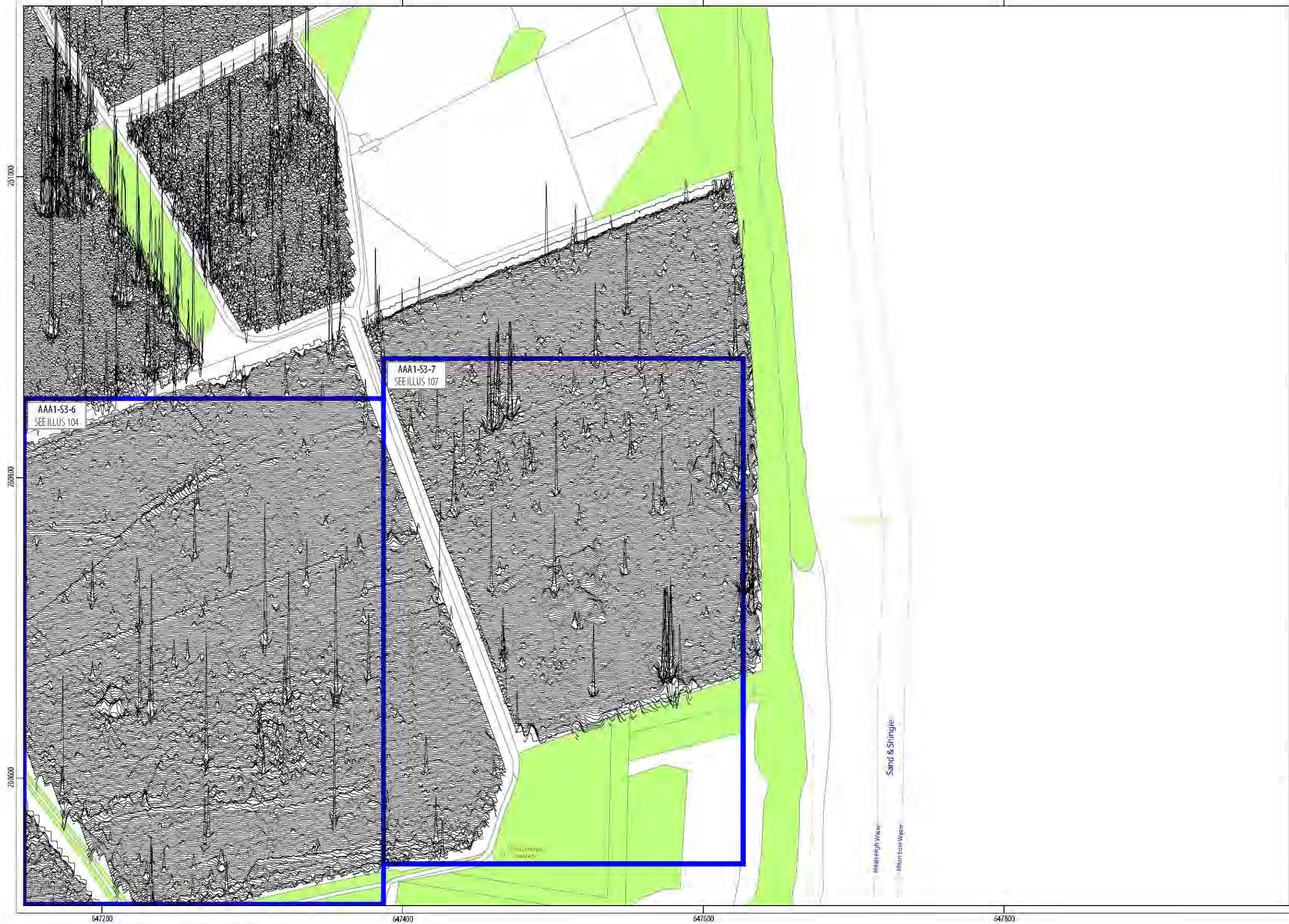
ILLUS 17 XY trace plot of minimally processed magnetometer data; Sector 3
