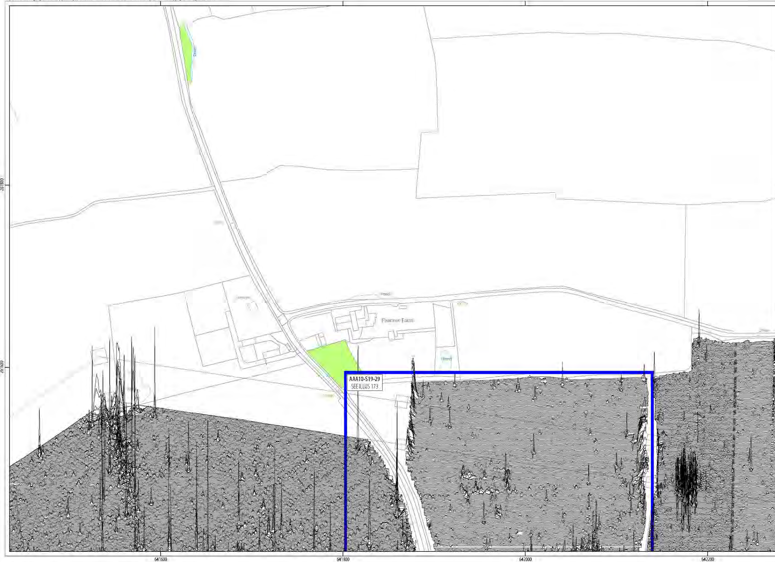
ILLUS 65 XY trace plot of minimally processed magnetometer data; Sector 19
