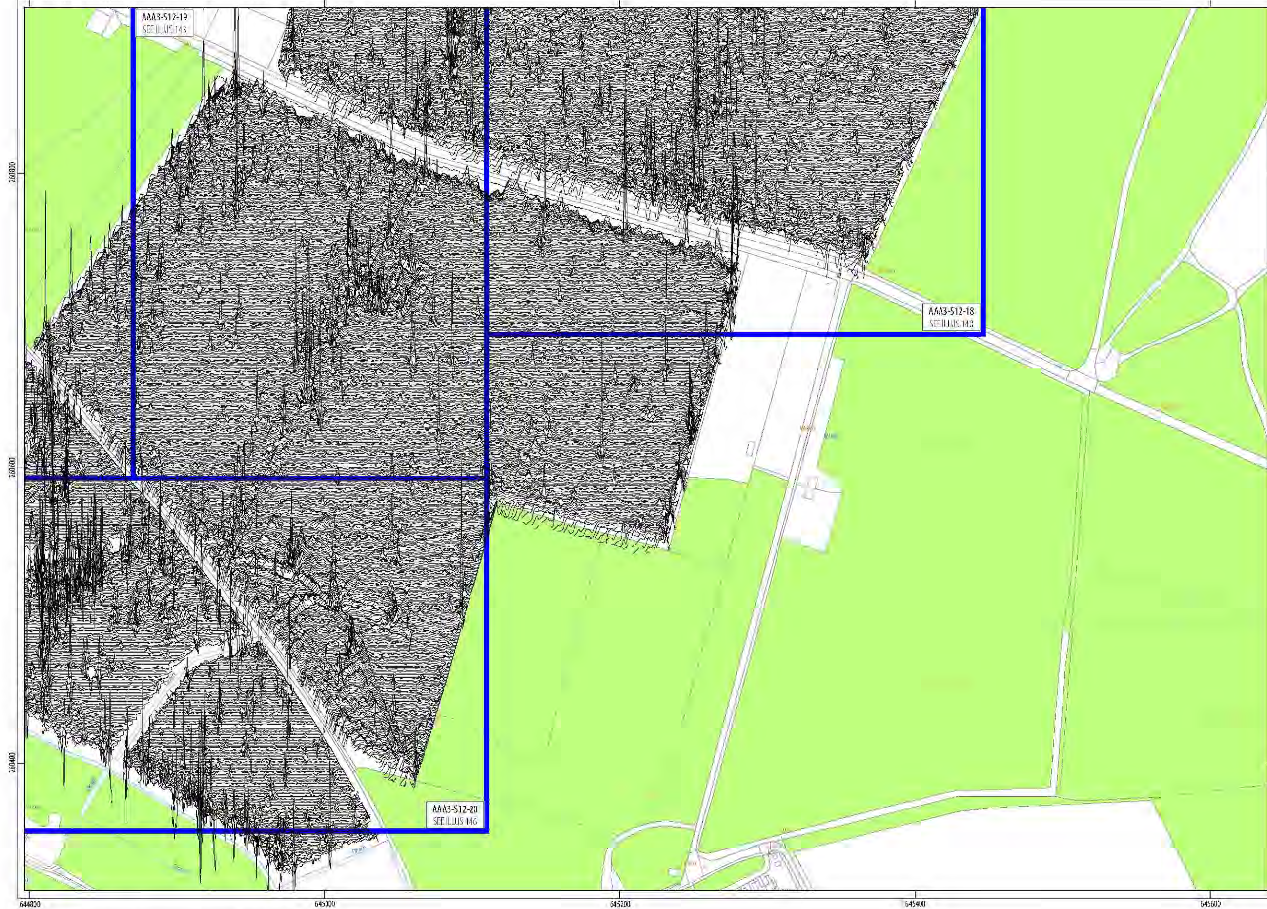
ILLUS 44 XY trace plot of minimally processed magnetometer data; Sector 12
